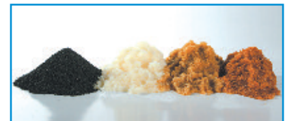
High grade materials are a vital aspect for highest quality. From left to right: Activated carbon, anions-, mixed bed- and cationexchange resins.
