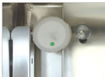
Gas supply line filter
